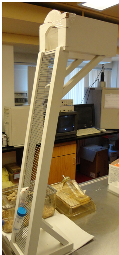
Fig. 2 Ladder. Inclined ladder ( 80^\circ ) with 100 \times 9 cm (length and width, respectively) used for the fatigue test. Falcon tube filled with water and attached to mouse tail
